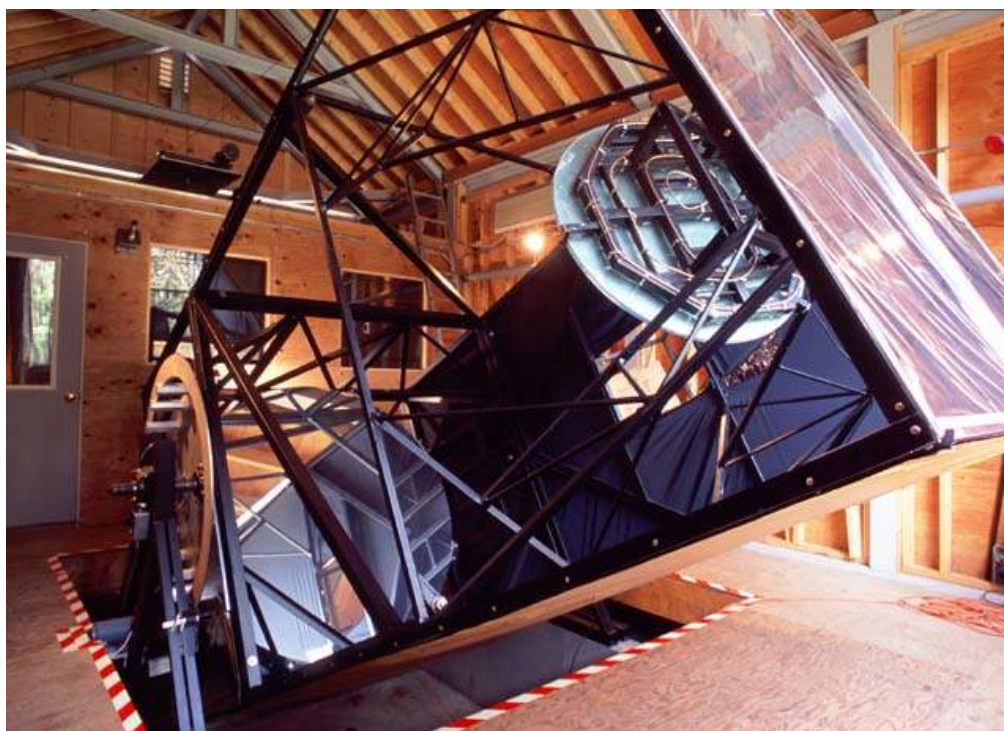
The Optical SETI telescope at the Oak Ridge Observatory in Harvard, Massachusetts. Note the unusual "boxlike" structure.
