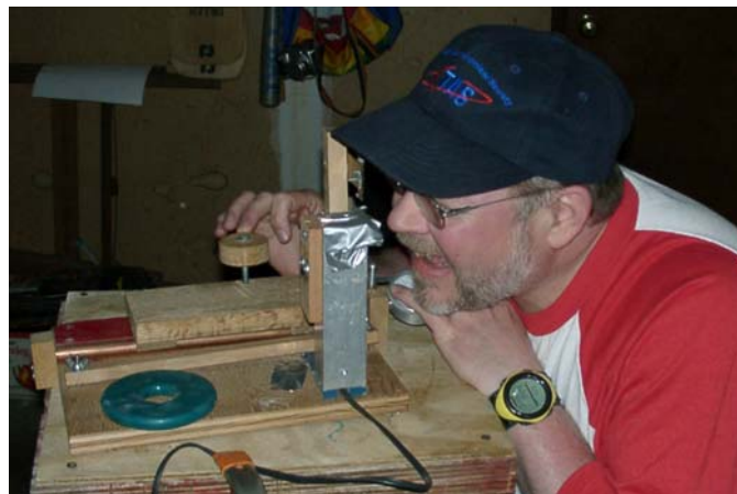
Bill Briggs measures results from the Foucault Knife test.
