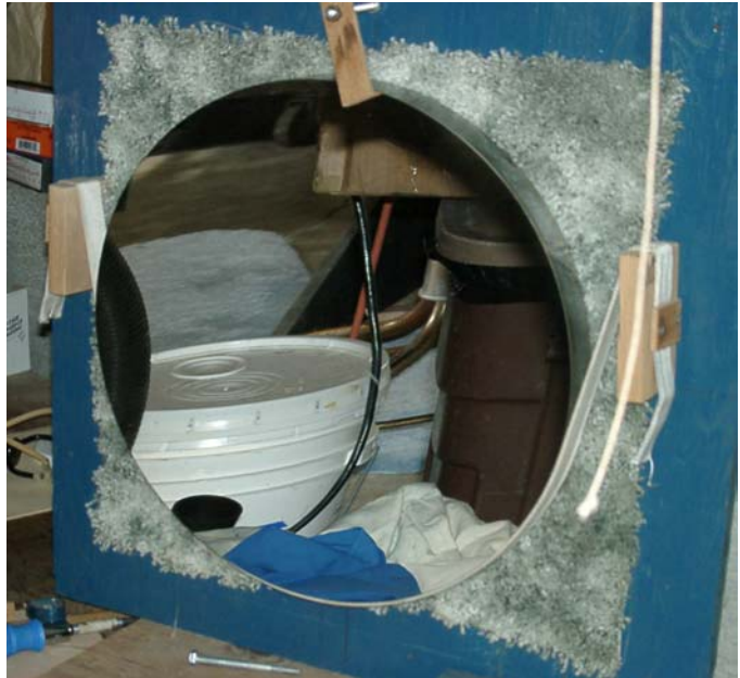
The 16" mirror mounted in a cradle ready for testing.
