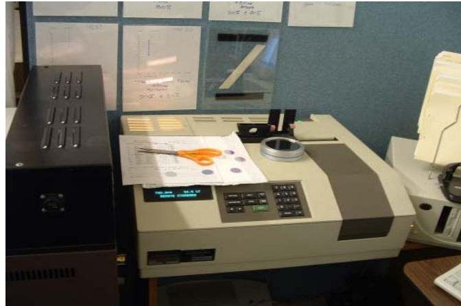
Spectrometer used for determining light absorption of coatings.
